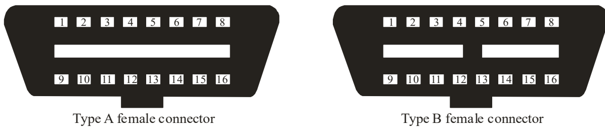
Fig. 4.1. The OBD connectors type A and type B. The type A connector is used for vehicles that use 12V supply voltage, whereas type B is used for 24V vehicles.
