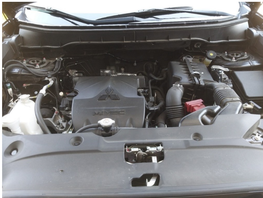
Fig. 2.1. Mitsubishi ASX engine MIVEC. It takes up a little space in the engine compartment.
