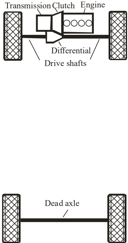
Fig. 1.2. Front-wheel drive (FWD) driveline architecture. Frequently transmission (gear box and differential) is named as one-unit transaxle [0.7, 0.13, 0.35]. The front of the car is at the top of figure.
